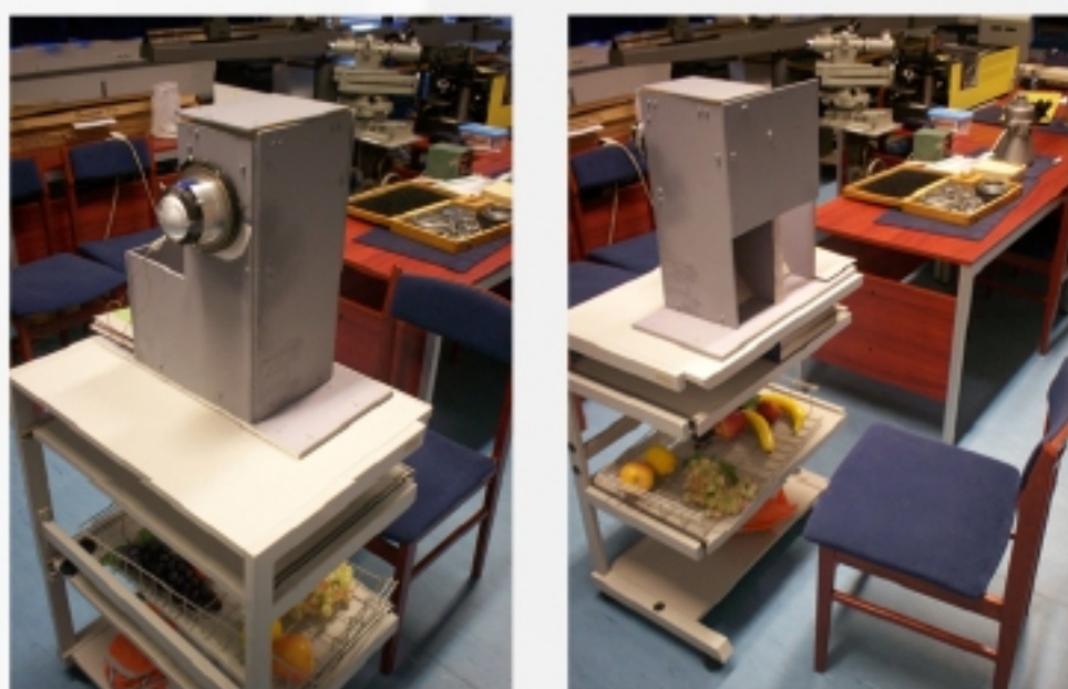
Fig.1. & 2. - Light booth for perceived brightness testing
