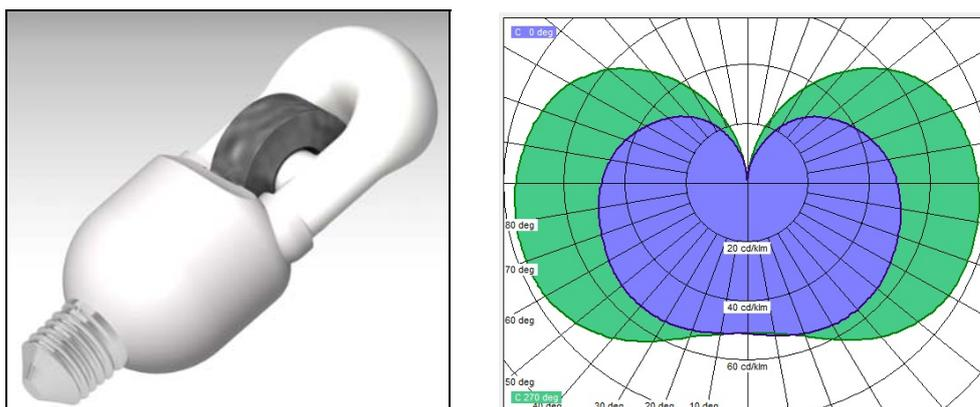
Fig. 1 Structure and luminous intensity distribution of the used induction light source
