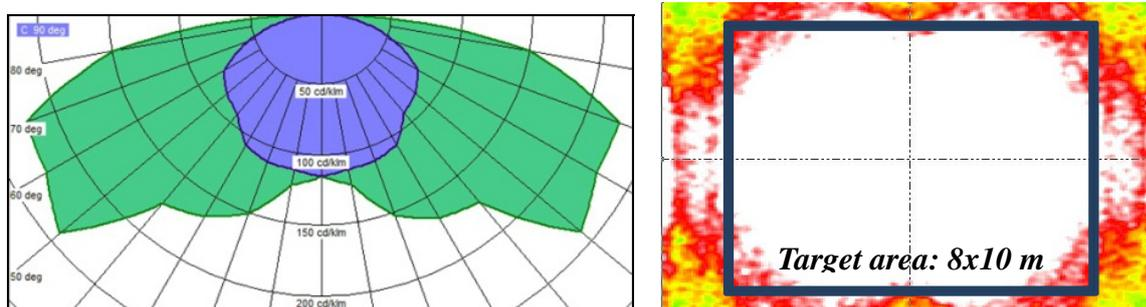
Fig. 4 Luminous intensity distribution (left) and illuminance results of the developed luminaire
