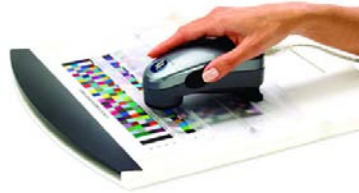
Fig.3. Calibration pattern and device using for calibration
