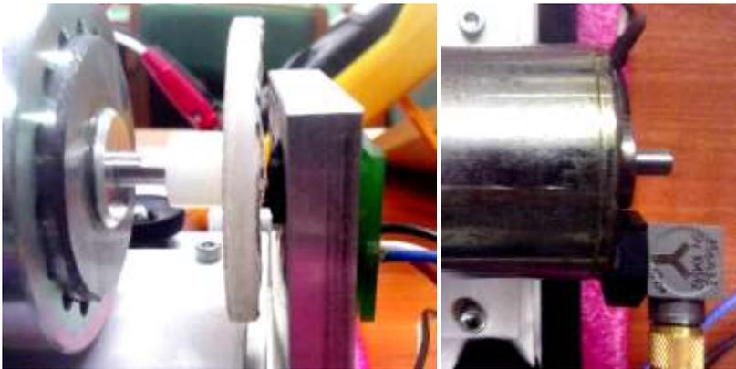
Fig. 1. Optical rotational speed measurement (left) and vibration measurement (right) of the analyzed system configuration
