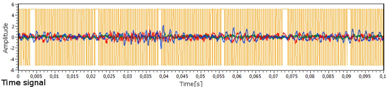
Fig. 3. Measured signals of optical sensor (yellow) and the 3D accelerometer (blue, red, green) at steady state of the system
