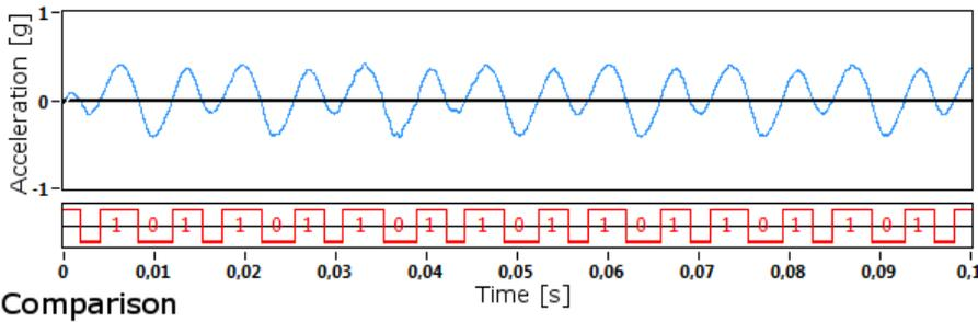
Fig. 4. Smoothed acceleration signal (above) and the compared beat diagram (below)
