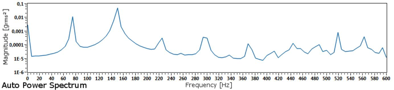
Fig. 6. APS of acceleration signal
