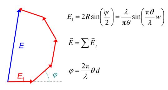
$$I = |\vec{E}|^2 = E_1^2 \left[ (1 + \cos \varphi + \cos 2\varphi + \dots + \cos(n-1)\varphi)^2 + (\sin \varphi + \sin 2\varphi + \dots + \sin(n-1)\varphi)^2 \right]$$
